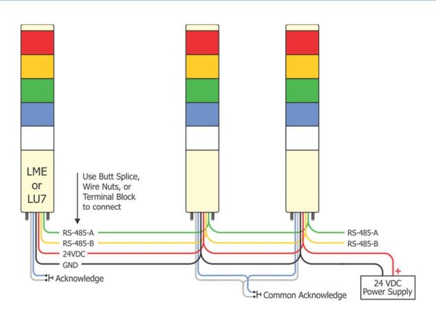
Multiple ACC RS-485 equipped LME and LU7 light towers can communicate with a computer or PLC over a common 4-wire network. Two of the wires are used for data and the other pair used for 24 VDC power. Since multiple towers operate over the same pair of wires, each has a unique address which is set using the configuration utility described later in this document.
