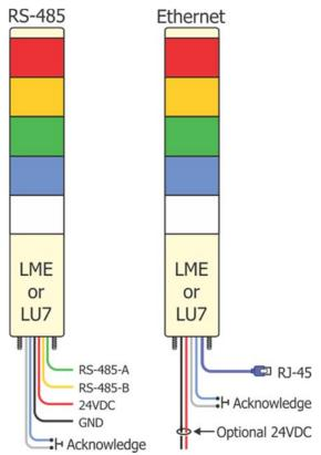
Two types of controllers are available. One communicates via Standard TCP/IP over Ethernet and the other uses an RS-485 balanced multi-drop network. The model numbers for these controllers are PA-06 for Ethernet and PA-05 for RS-485.
